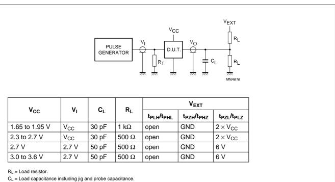
$R_T$  = Termination resistance should be equal to the output impedance  $Z_o$  of the pulse generator.
